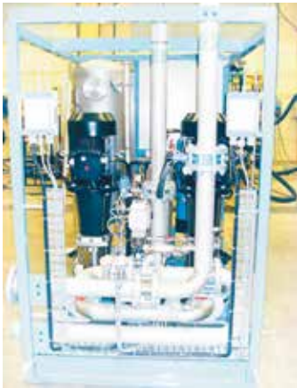
Cooling water pump unit
